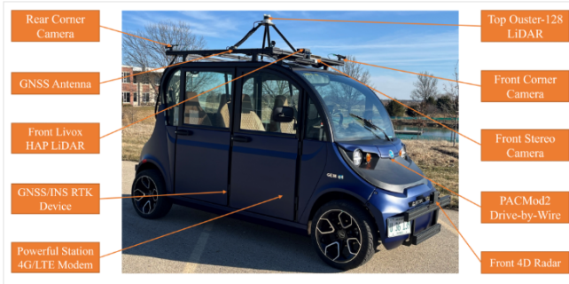
Fig. 2: GEM vehicle platform sensor and compute stack.
